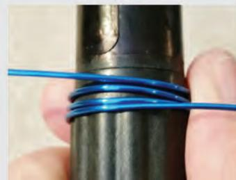
3. Cross over the two wires so that they link together.
